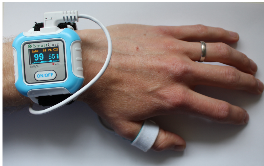
Figure 2.2: Smartwatch-like device used by Charlton, SmartCare wrist-worn pulse Oximeter [8, Figure 1]
