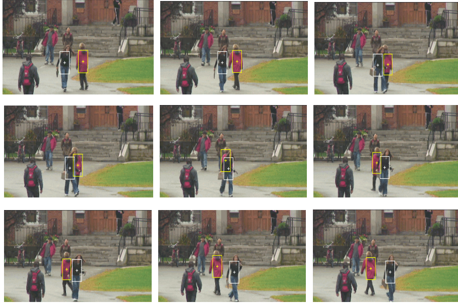
Fig. 1. First row: Tracking during the pre-occlusion phase. Second row: Tracking during the occlusion phase. Third row: Tracking during the post-occlusion phase.
