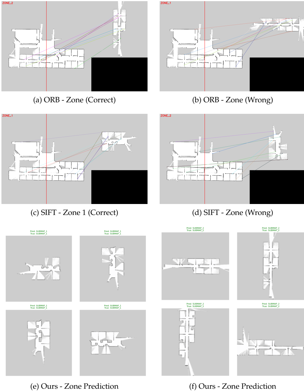
Figure 4.6: Visual comparison of ORB, SIFT, and our GoogLeNet-based approach in zone classification. Correct and incorrect predictions are shown for traditional methods, while our model provides consistent results.
